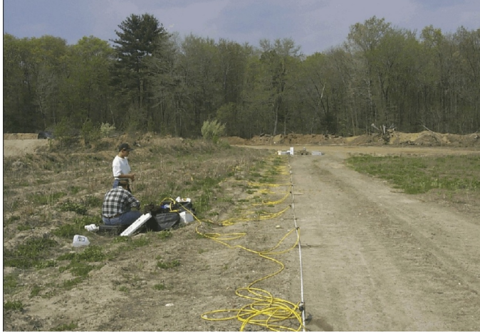
Figure 1.1. DC resistivity survey. Current is injected into the ground and potentials are measured above the ground or in boreholes. The goal is to estimate the contaminated plum.
